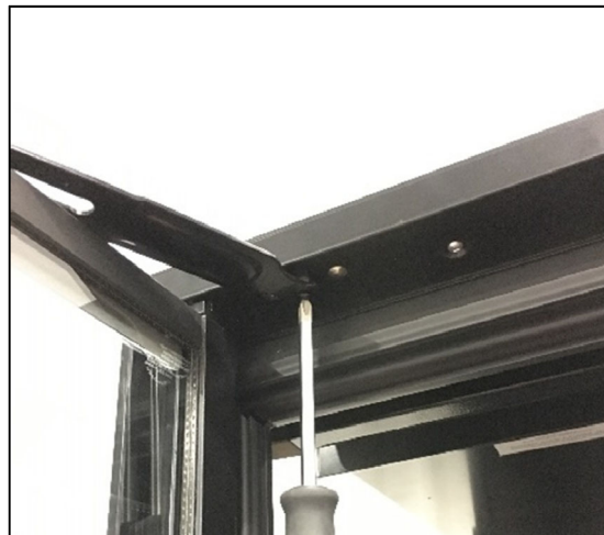
Figure 13. Remove Hold Open Screw
